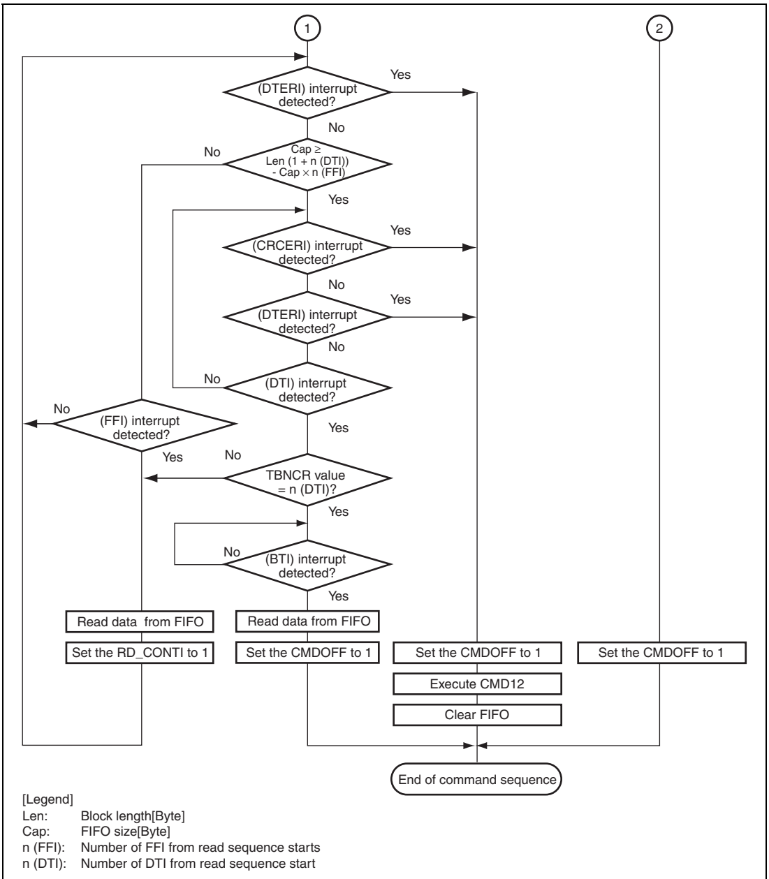
Figure 24.13 Example of Operational Flow for Commands with Read Data (4) (Pre-defined Multiple Block Transfer)
